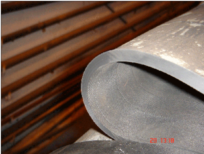
12mm thick vulcanized rubber coating
