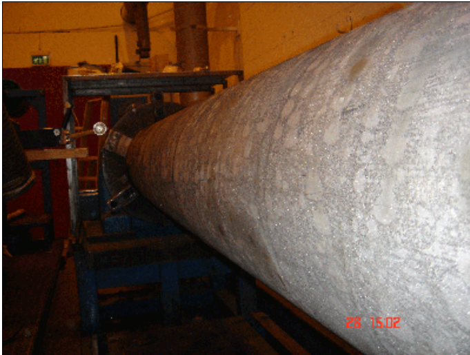
Completed (cleaned ) pipe on rotating lathe bed
