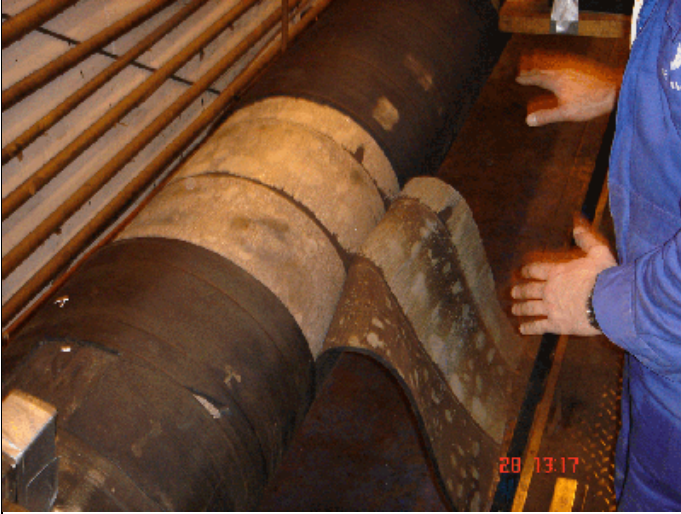
Vulcanized coating is easily removed
